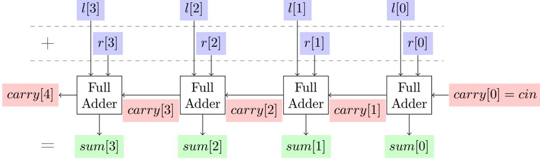
Figure 3: Ripple-carry adder, combining multiple full adder circuits to add bit vectors of arbitrary size.
