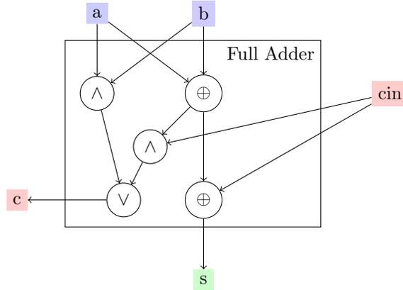
Figure 2: Full adder circuit, adding two bits together while considering an incoming carry and producing a result and outgoing carry bit.
